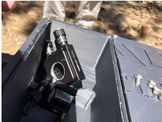
Figure 17: Optics Damage Due to Drop
